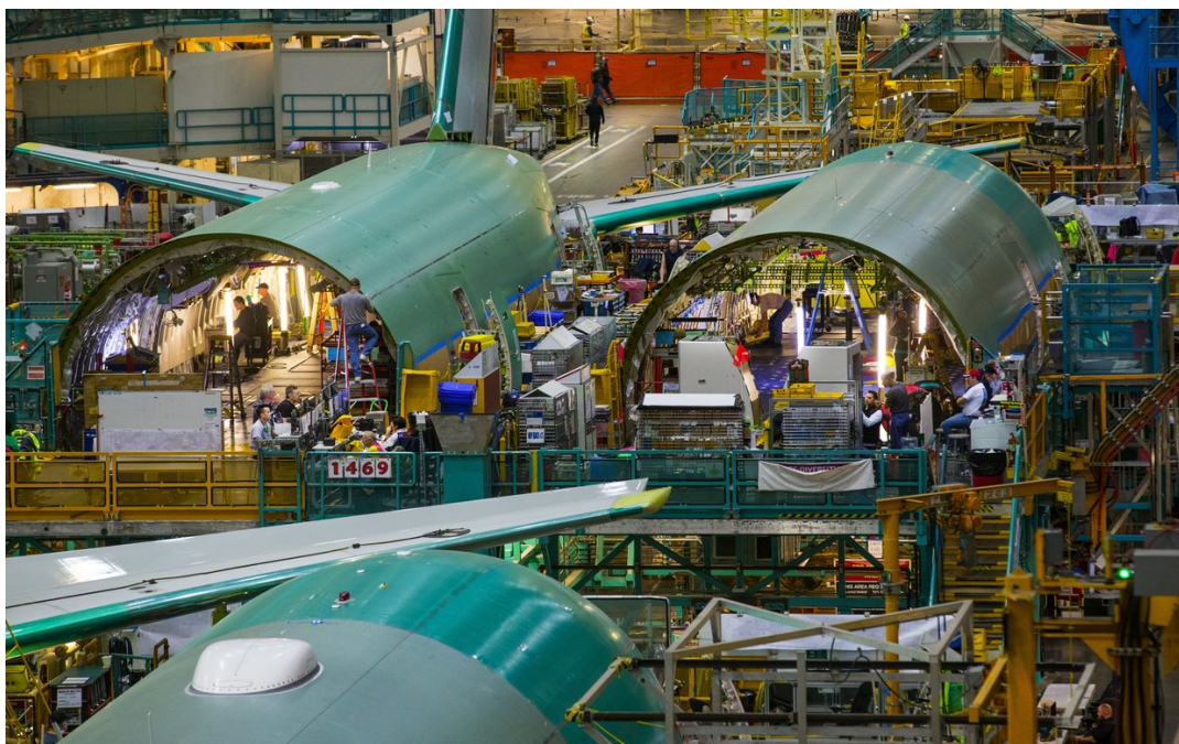
Boeing 777 fuselage sections in various stages of production, at Everett's final assembly line. The assembly line is being re-configured in preparation for 777X. Photo taken Dec. 9, 2016. (Mike Siegel/The Seattle Times)
